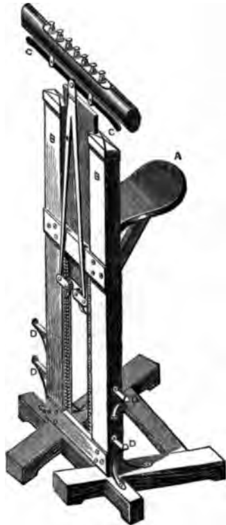
OBSERVING CHAIR, DEVISED BY E. B. KNOBEL.
